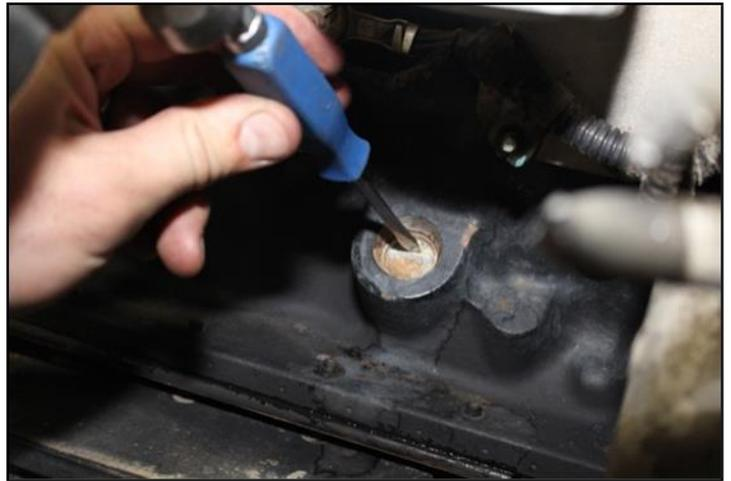
***NOTE:*** Be sure to clean around the freeze plug and remove all debris from the cup of the freeze plug to make sure nothing drops into the oil pan. **Be very careful not to push the plug into the oil pan, or you will have to drop the oil pan to retrieve it.**
