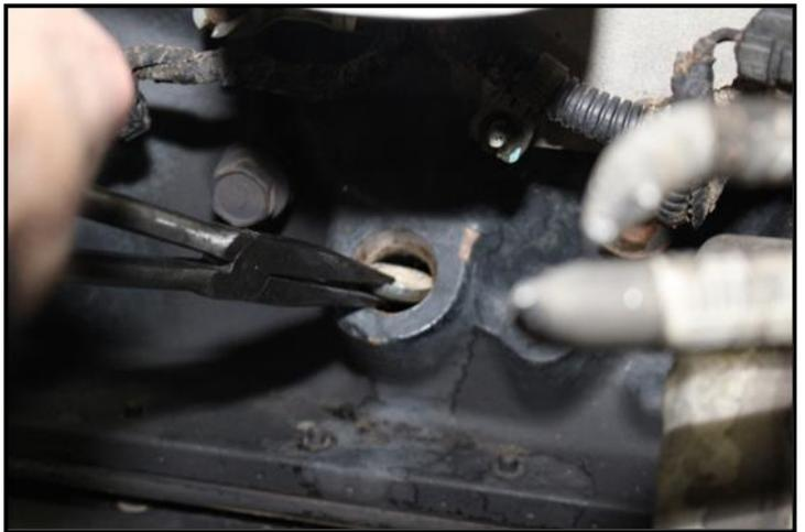
17. Remove the rear factory oil drain from the block. Insert the provided long oil drain line into the front drain port and short oil drain line in the rear hole (where factory drain line was connected). **Keep drain lines as straight as possible while pushing them into the holes, so you do not damage them.** Make sure they are pushed completely into the hole. Both O-rings should be inside the hole. The long oil drain line will be connected to the top turbo later as shown.
