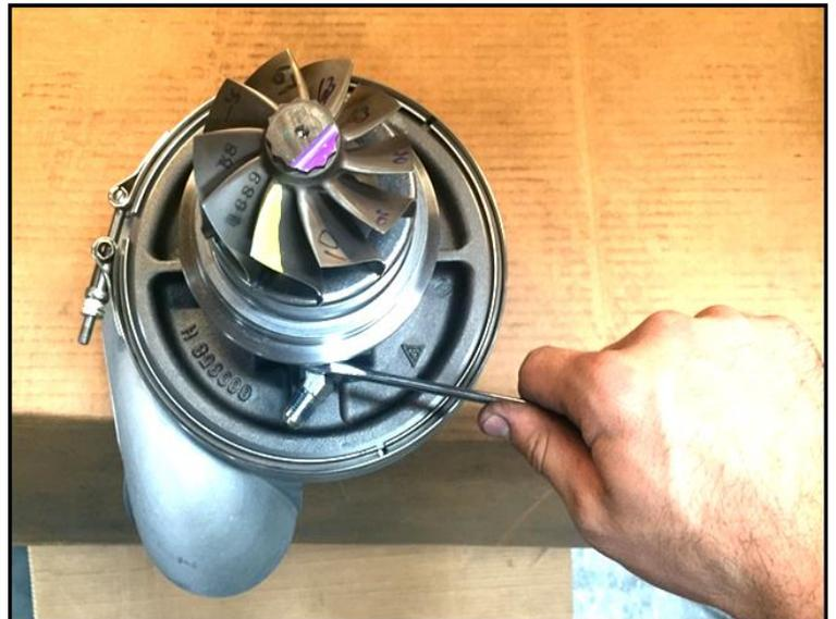
30. Install oil supply line (steel braided hose without elbows) to the oil inlet elbow fitting on large turbo as shown. Tighten the fitting snug, but do not over tighten.
