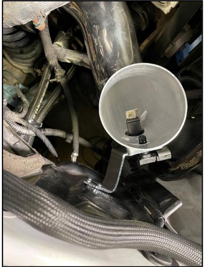
41. Once again check to make sure that all tubes, cords, and lines are not in contact with any portion of the Compound Turbo Kit.
